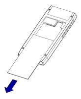
3. If the battery is inserted, remove the battery as show.
