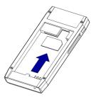
5. Replace the battery as shown, with the contacts of the battery aligned with the corresponding connectors.
